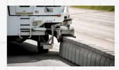
One-meter sections of highly reinforced concrete barriers are pinned together at each end to form a continuous barrier wall. The barriers have a "T" top, which acts as a lifting surface for The Road Zipper Machine.
