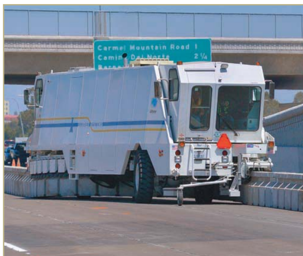
The Barrier Transfer Machine changes the moveable median barriers to accommodate the flow of traffic.
