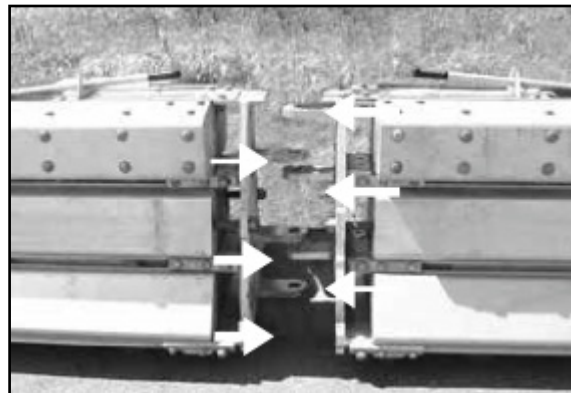
Figure 7. There are two different ends on a barrier section. Be sure that you have a Lower hinge matched with an Upper hinge section before installing the hinge pin.
