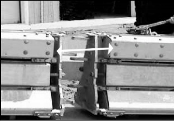
Figure 16. Use a winch or a “come along” as shown above to bring two sections together on a slope so that the hinge pin can be removed or installed.
