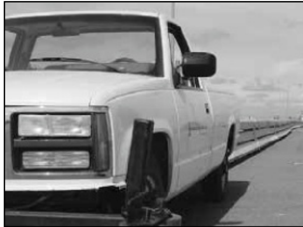
Figure 17. Pull the barrier straight or at an angle. For an angled move, all of the steering wheels (using the tiller handle) must be positioned in the desired direction. Always use caution when towing large sections of barrier.
