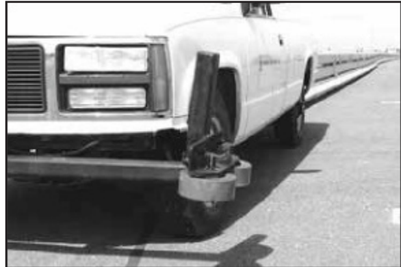
Figure 12: The push rollers move the barrier sections without causing damage.
