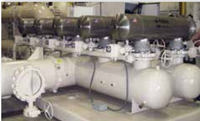
The pump station was custom-engineered and performance-tested, as shown above, at the Watertronics facility in Hartland, Wisconsin, USA.
