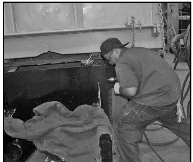
Figure 5. Drill holes through the frame rails.
