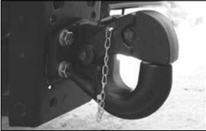
Figure 8. Use a correctly rated pintle hook
