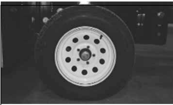
Figure 20. Check tire pressure and lug torque
