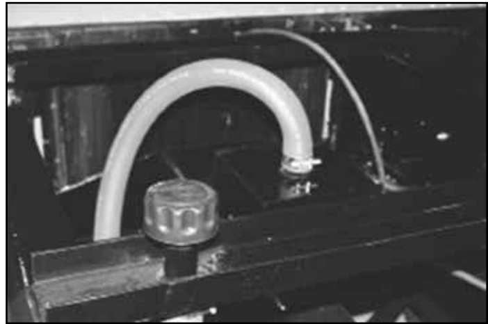
Figure 21. Check hydraulic fluid
