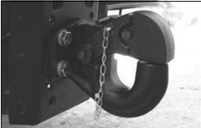
Figure 25. Check for correctly rated pintle hook
