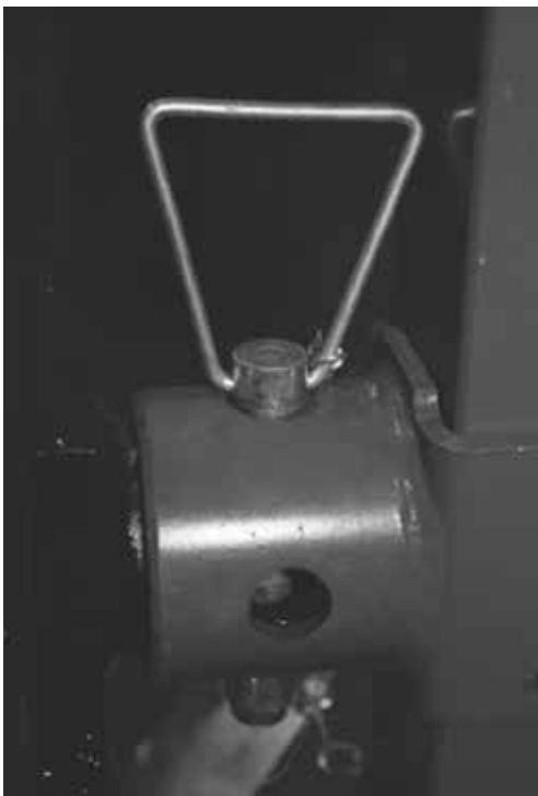
Figure 19. The jack pin is engaged
