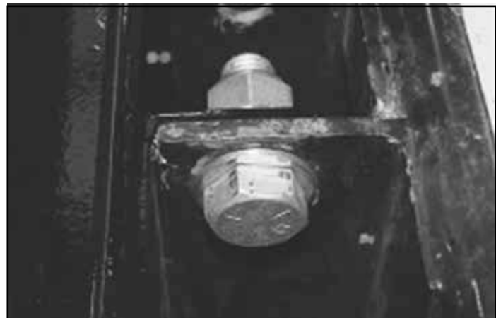
Figure 22. Check torque on mounting nuts
