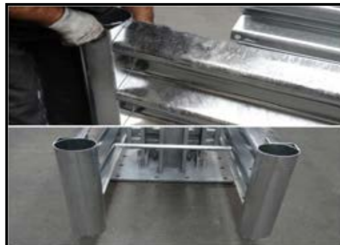
Figure 15 Mounting end tube
