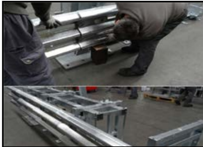
Figure 10a Mounting of the panels and of the sliders
