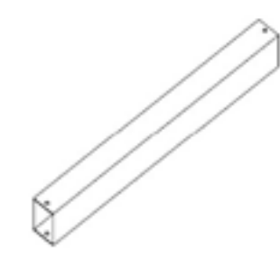
Tube 80x80x2 L=920 TUB0007
