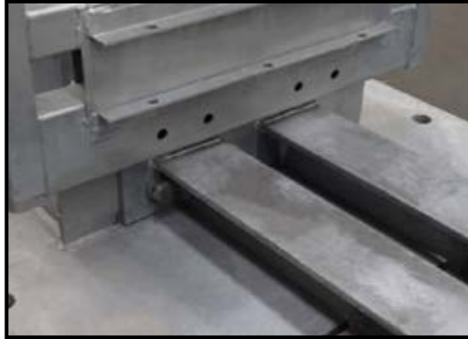
Figure 3a Fixing rails to backstop
