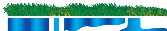
Drip irrigation – uneven and interrupted application due to clogging and rodent damage
